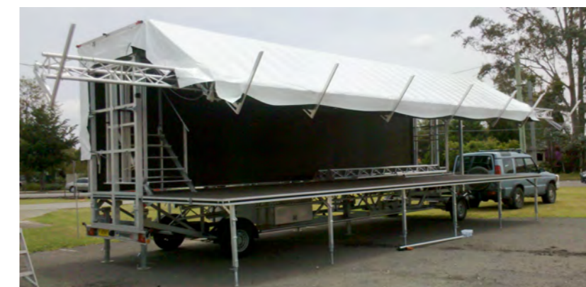
Over Stage Banner Holders are accessible easily during stage assembly. Image shows full width including PA wing holders. Also visible is the velcro attachment location for the banner as a Stage Skirt.
